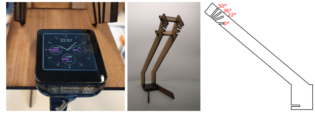
Figure 2: Left: The Sony Smartwatch 3 used in all three studies. Middle: Our custom-made study stand. Right: The angles we used in the study represented on a sketch of our study stand.
