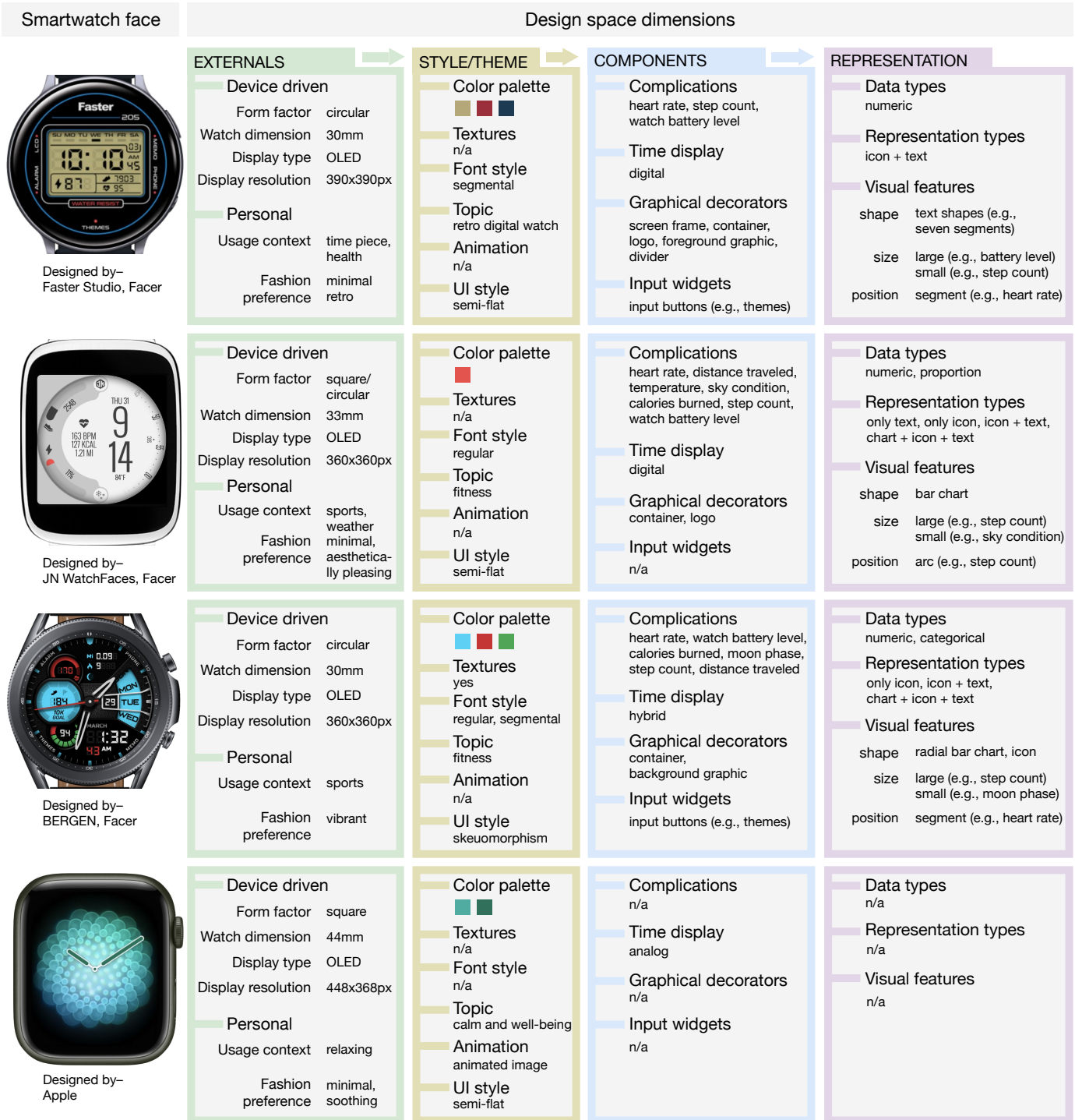
Fig. 7: Four examples of smartwatch faces using our design space dimensions to describe them.
